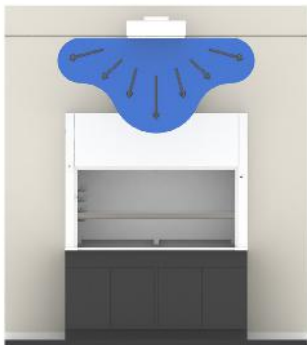
TriTec Laboratory Application - End View
